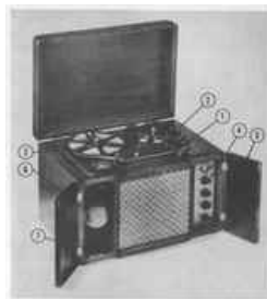
FIG. 6-48. BK-411 Soundmirror. This instrument has a single knob (1) to control all mechanical operations, such as slow forward speed of 7.5 in. per sec. for recording and reproducing, fast rewind speed to return the tape from the take-up reel (2) to the supply reel (3), and fast forward speed to find promptly any desired part of the recorded program. The 7-inch reels hold more than 30 mm. of recording. All electronic functions are controlled by the four knobs (4), which can be hidden by closing door (5). Microphone (6) can be stored in special compartment (7). (Courtesy of The Brush Development Company.)
