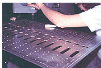
Machining console panels
