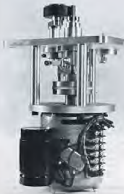
Capstan drive sub-assembly removed from top-plate.
