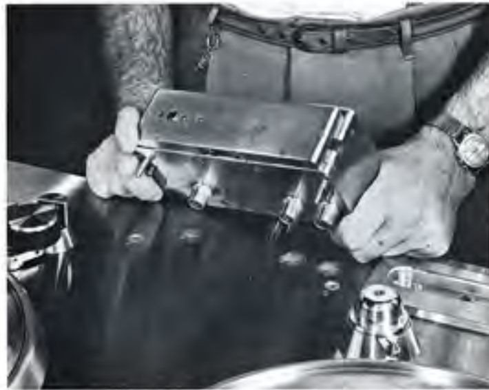
View illustrating plug-in feature of magnetic head assembly. Slotted cap screw at left of head gate covers hole for editing pencil insertion over playback gap.
