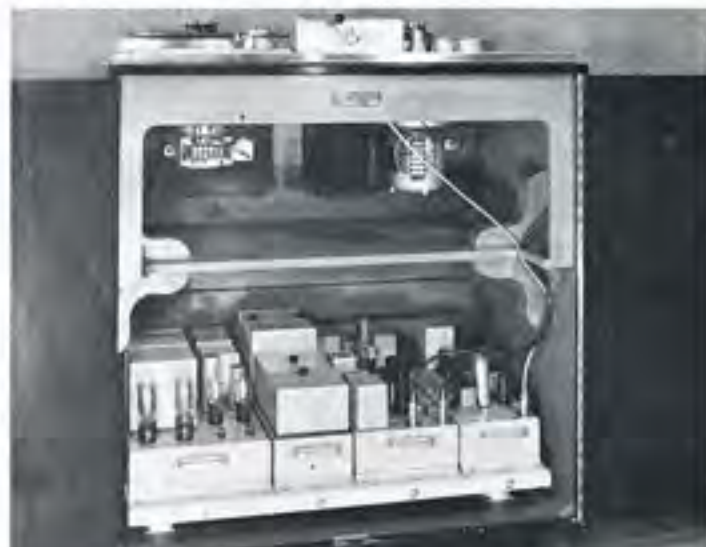
Front view with cabinet doors opened. Note modular electronic assembly on vibration-isolated base. Removable modules are (left to right) power supply, control logic assembly, record module, and playback module.
