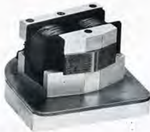
Original prototype Ampex playback head (enlarged 3.5X). This is the actual head that was proportioned to allow mounting in Mullin's Magnetophon head housing for proof of performance.
