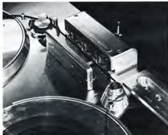
Partial view of top-plate showing cast Meehanite head housing with gate forcibly extended beyond its regular open position permitting view of magnetic heads. Note alloy inner shield cans. Far left head is play-back with laminated shield can. Also shows straight-line threading path of tape.
