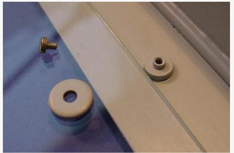
Detail of the construction to keep the glass aligned and fixed in the frame (screw = M2)
