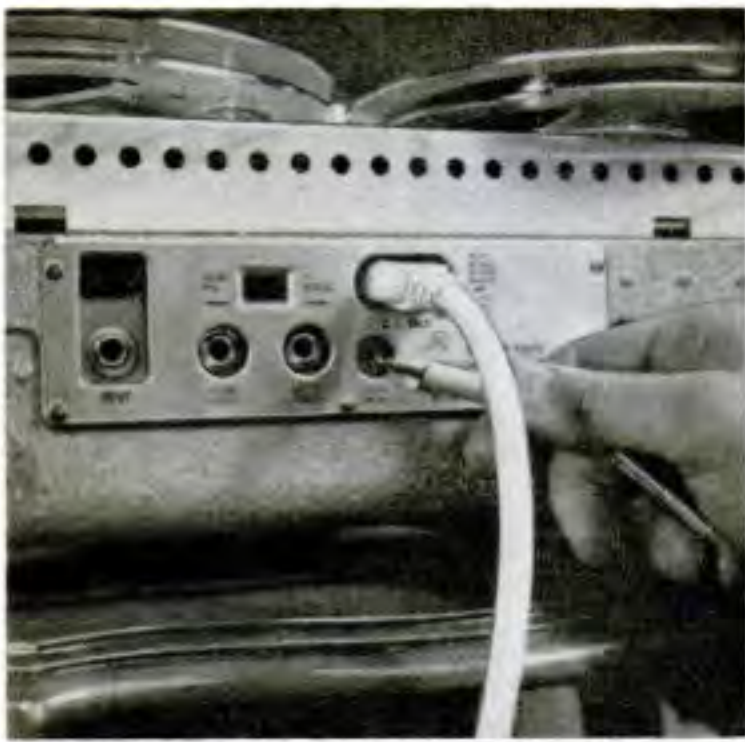
Wollensak model 1616 shown here requires an external amplifier and speaker for second channel
