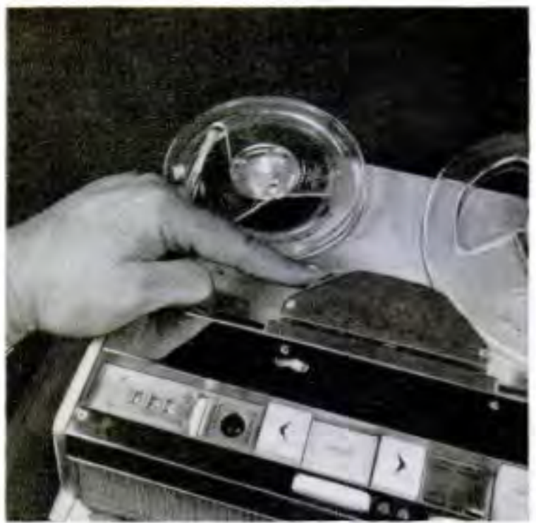
Many tape recorders have shift levers to select either half-track or quarter-track arrangement
