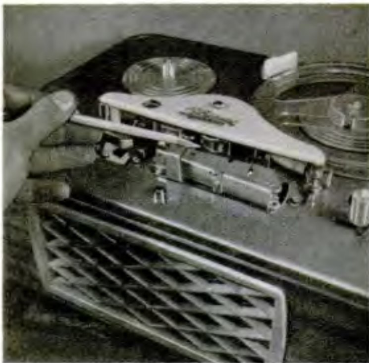
Fixed position heads such as on the Tandberg produce only half-track tapes and play them as well
