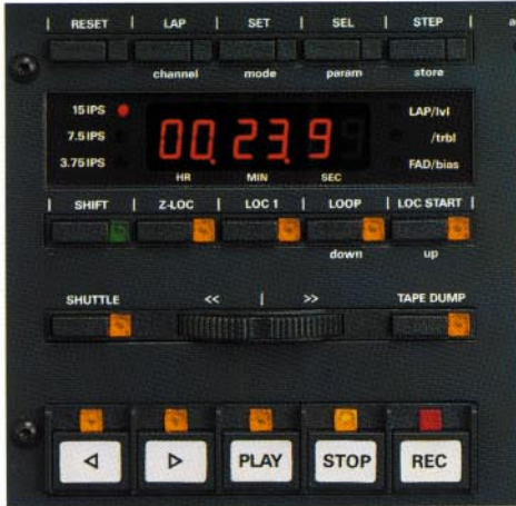
Tape timer and tape deck functions of the STUDER A807 family.
