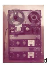
Roberts 997. Based on an Ampex 600-2. Tube electronics. Really enjoyed this machine. A little finicky, but very easy to work on.
