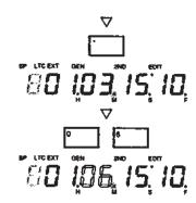
After correcting the time data, press the STO key, and selected n (using the numerical keypad), to store into cue memory "n".
