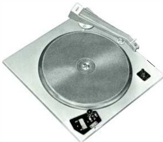
CB-510 complete operating transcription turntable includes CB-500 low noise chassis with synchronous motor, GRAY 208-S/G viscous damped pickup arm, twin flip-over 1 mil and 3 mil reluctance cartridge, 2-position variable equalizer to NAB/RIAA and high frequency roll off curves and M-6244 transistorized preamplifier with self-contained power supply. Output: 150 or 600 ohms adjustable from -22 dbm to -12 dbm, 12 MV input.
