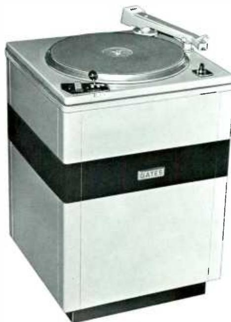
CB-525 and CB-525A turntable. This is the same as the CB-510 turntable but with the CAB-6 floor cabinet added. CAB-6 cabinet has adjustable leveling screws, full size rear door. Made of 5-ply seasoned birch, sealed and finished in gloss gray and black. Size: 21 $\frac{1}{4}$ " wide, 21 $\frac{1}{4}$ " deep, 29 $\frac{1}{2}$ " high plus 1" for leveling screws. For CB-500 chassis or CB-510 complete turntable.
