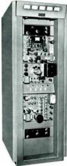
The Gates BT-100C is the most outstanding new television transmitter developed in the United States during the past five years. The transmitter was designed especially for the CCIR 625 line standards and for operation with 50 cycle power source. The BT-100C is field proven at overseas locations, including the tropics, operating on CCIR standards. When operated on U.S. 525 line standard on 60 cycle power the BT-100C is rated very conservatively at 120 watts peak visual power.
