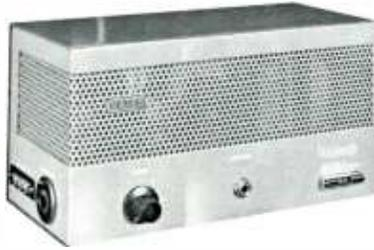
The M-5531 Unimote will perform equally well as a microphone preamplifier, turntable preamplifier, program amplifier up to 18 dbm output, repeater amplifier, isolation amplifier or as a standby amplifier for quick connection to an emergency circuit. The cover is easily removable for 100% accessibility by flipping two snap locks. Includes front panel gain control and Cannon XL-3 connector.
