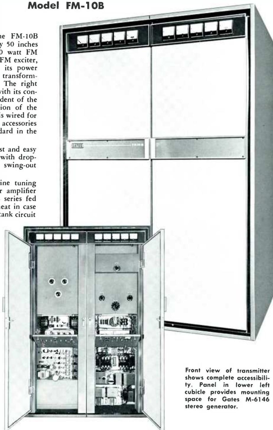
Front view of transmitter shows complete accessibility. Panel in lower left cubicle provides mounting space for Gates M-6146 stereo generator.
