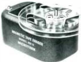
Bulk tape demagnetizer developing high intensity magnetic field. Erases recorded signals and noise completely and restores tape to like new condition. Handles 5", 7" and 10 1/2" reels. Adapter hub available (optional accessory) for 10 1/2" reels. 117 volts, 50/60 cycles.
