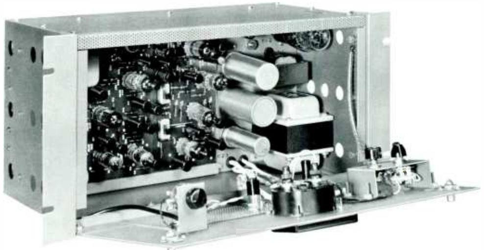
Hinged-down front panel permits complete front accessibility of components and inner servicing adjustments. Printed wiring by the Gates solid adhesion process assures uniformity and ease in both cleaning and circuit analysis. "Level Devil" finish is a medium gloss gray over a heavy prime coat. Design is for continuous duty.
