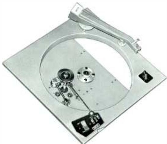
CB-510 turntable with platter removed showing the shift mechanism. The transistorized preamplifier bolts to the under side of the turntable chassis and has its own self-contained silicon power supply.
