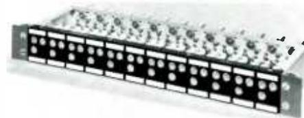
For patching coaxial circuits. 12 groups of 3 jacks on a strip 2 1/8" x 19". Contacts heat treated beryllium copper. Outer braid of coaxial cable may be soldered directly to jacks for complete shielding. Patch cords and plugs listed and illustrated below.
