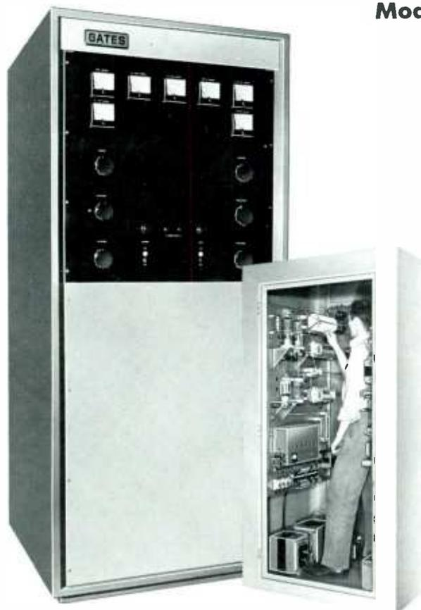
Fully FCC type approved, the Gates BC-250GY is the most widely used 250 watt AM broadcast transmitter and has a world-wide reputation for long trouble-free service. It consists of three audio frequency stages with provision for 2 crystals in temperature controlled ovens. The Type 813 RF driver provides an abundance of drive and long tube life. A pair of Type 810 single ended power amplifiers feed an output coupling network that will match specified impedances from 30 to 300 ohms.
