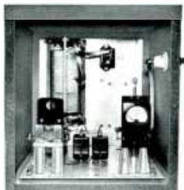
A fully weatherproof coupler for series feed antennas to handle 1250 watts or less and at 100% modulation. Meter shorting switch is provided in antenna circuit to eliminate damage to meter during electrical disturbances. Antenna meter may be observed through glass porthole. Coil is silver plated, having generous inductance for arrangement in a full Tee network along with the fixed mica capacitors supplied. Extra room is provided in the cabinet for either
