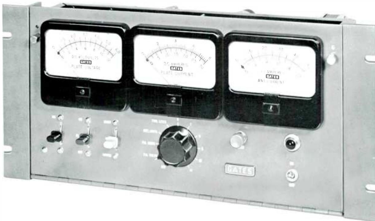
The RDC-10AC meets FCC requirements for remote control of AM and FM broadcast transmitters. It is the most widely used control system for unattended operations.
