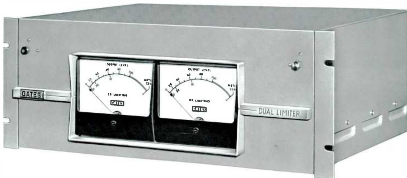
FM stereo broadcasting has created the need for specialized audio equipment. Of major importance is the stereo limiting amplifier. The content of a stereo signal is such that two individual single channel limiting amplifiers will not provide best service. The difference in level between stereo channels may cause one channel to limit heavily while the other is not limiting at all. This will cause unbalance between channels and serious loss of stereo effect.
