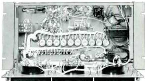
Studio unit has drop-down front panel so all parts can be reached from front of rack. Panel size of 8 3/4" x 19" conserves much needed rack panel space.
