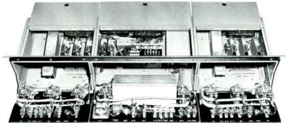
mounted in sturdy cast aluminum housings with interconnecting cables and plugs.
