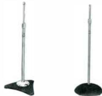
A floor stand with a big heavy base, listed to left above. Weight 24 lbs., and base 17" across. Adjustable to 66". Full chrome with gray base. 3/8" x 27 thread. Non-slipping clutch. Fits all microphones listed in this catalog.
