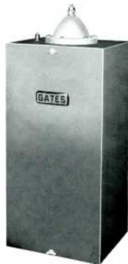
**Model M-5178:** Series feed, provides all coil capacitance to provide full Tee network. Constructed in non-weatherproof steel cabinet, front removable. Size: 21" high, 10" wide, 9" deep. Matches RF input of 50 or 70 ohms. Output 10-600 ohms. In this model metering is external to the coupler, often desirable in unattended operation. For all powers 100% modulated up to 1250 watts carrier.
