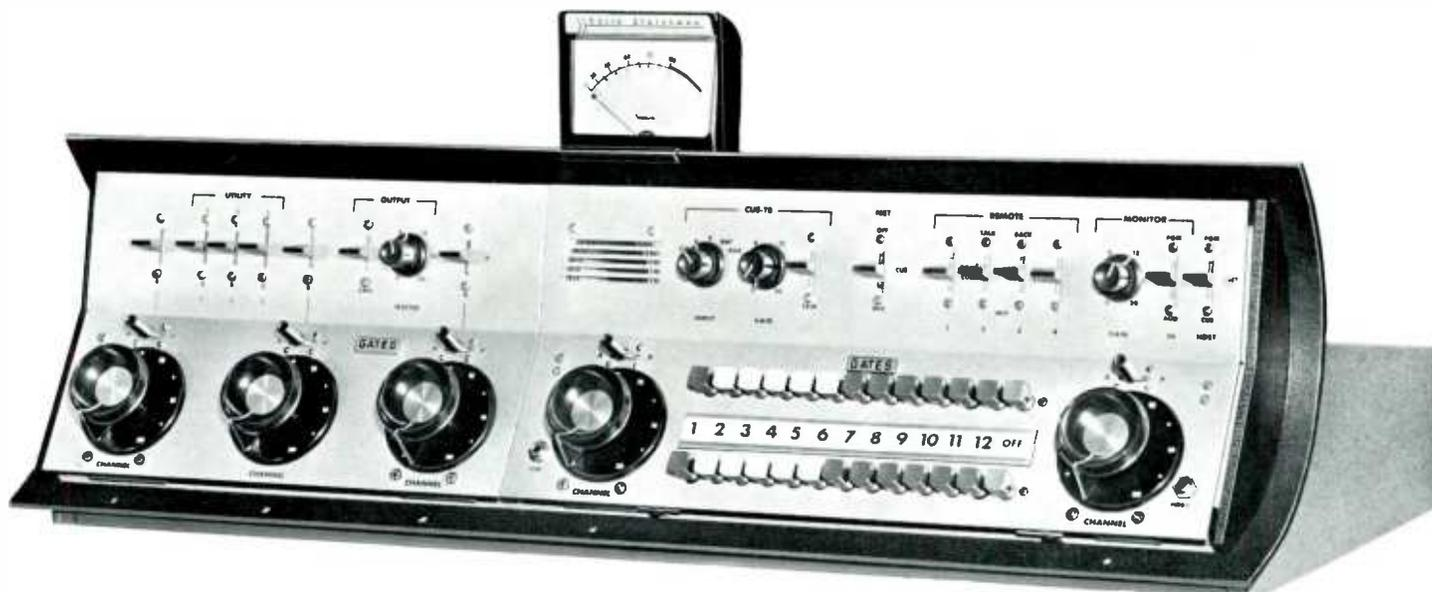
The *Ambassador* is a completely transistorized 5-channel audio control console.
