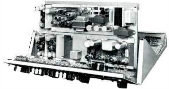
Studioette top cover is completely removed. Front panel hinges out to reach every "behind the panel" component. The amplifier deck hinges up so that muting relay contacts are at finger tip when touch-up burnishing is required.
