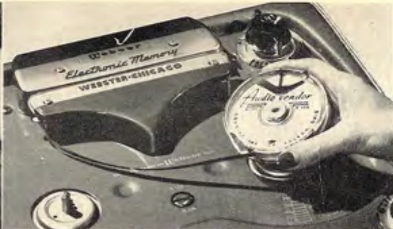
Left: among cartridge developments is the Mini-Music made by the Television Associates of Indiana which appeared in 1951. The small plastic container held a continuous loop of tape. Right: the Cousino Audio Vendor uses graphite lubricated tape in a moebius loop. Both devices are used for talking displays and similar applications.
