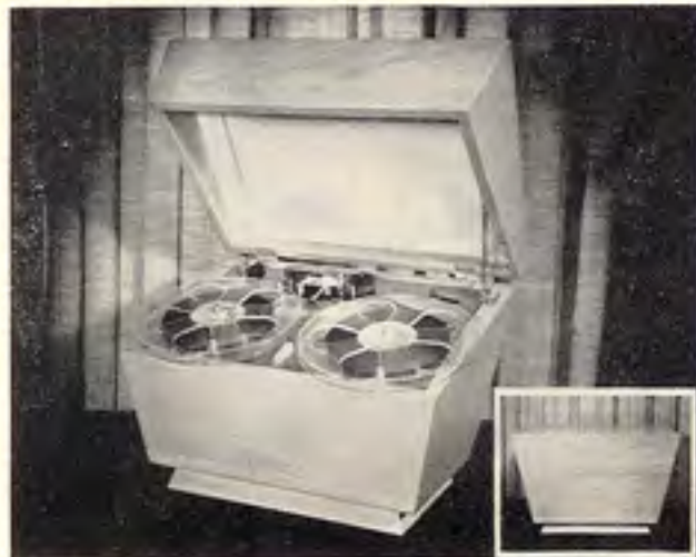
Left: the Pentron electronic orchestra. This unit had six separate channels on 1/4 inch tape, one for each of the six instruments in the band. It was shown in 1953. Right: a reproduction of the first stereo tape catalog. This single sheet was put out by Livingston in May 1954. Below: Livingston designed and sold this stereo player, the first on the market to provide something for the public to play its tapes on. It had staggered heads, as had the first Magnecords.
