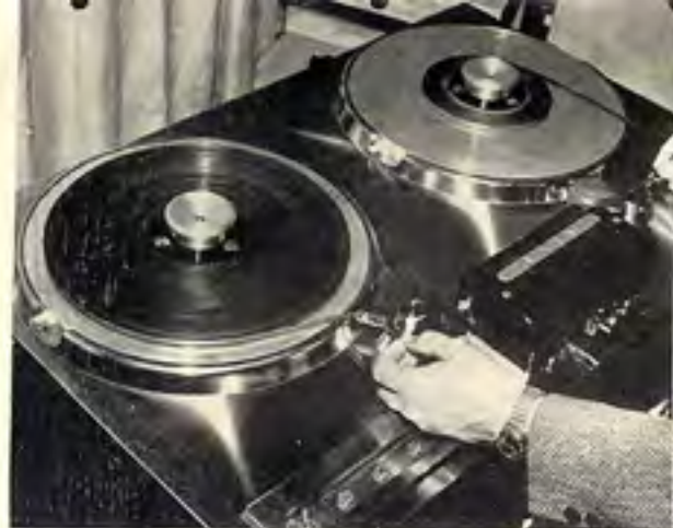
Left: this is an Ampex 200 tape recorder patterned after the German "Magnetophon" which used a special Minnesota Mining and Manufacturing Co. tape—No. 112—which was introduced in April of 1948. Subsequent Ampex recorders were modified to utilize 3M's red oxide tape No. 111. Tape speed of the Ampex 200, like the German "Magnetophon," was 30 inches per second. Right: tape recorder which was instrumental in switching the hundreds of radio stations over the country over to magnetic tape was the "Magnecorder" shown here, brought out in 1948. Magnecorder started making professional wire recorders in 1946 but switched to tape.
