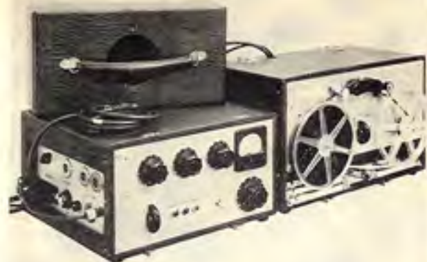
Left: this is an Ampex 200 tape recorder patterned after the German "Magnetophon" which used a special Minnesota Mining and Manufacturing Co. tape—No. 112—which was introduced in April of 1948. Subsequent Ampex recorders were modified to utilize 3M's red oxide tape No. 111. Tape speed of the Ampex 200, like the German "Magnetophon," was 30 inches per second. Right: tape recorder which was instrumental in switching the hundreds of radio stations over the country over to magnetic tape was the "Magnecorder" shown here, brought out in 1948. Magnecorder started making professional wire recorders in 1946 but switched to tape.
