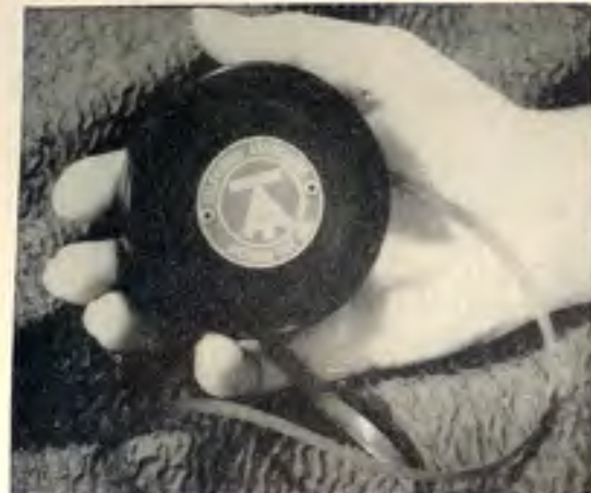
Left: among cartridge developments is the Mini-Music made by the Television Associates of Indiana which appeared in 1951. The small plastic container held a continuous loop of tape. Right: the Cousino Audio Vendor uses graphite lubricated tape in a moebius loop. Both devices are used for talking displays and similar applications.
