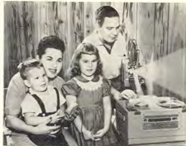
Left: the Revere Camera Company of Chicago developed its Synchrotape to permit more accurate synchronization of sound from tape with home movies. The tape was striped and the flicker of the projector shutter provided a stroboscopic light effect to time the recorder and projector. Adjustments in speed were made manually. Right: automatic control of slides for home and business was provided by this Model 207 Ekotape. The top track of the tape was used for voice or music and the lower track for signals which, through a relay, operated a slide projector and changed pictures without an operator touching the controls. Earlier devices included a photo cell mounted on a recorder which picked up the light reflected from white tabs attached to the back of the tape.
