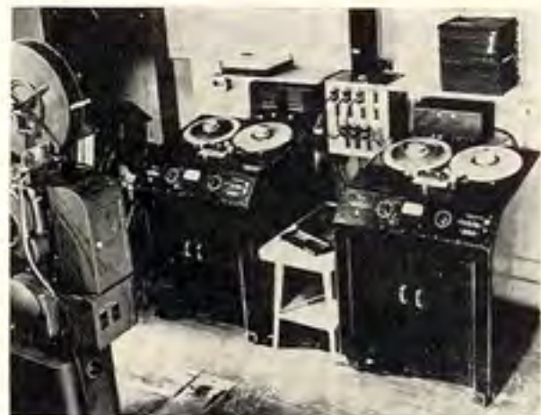
In use by 1949 were these Fairchild professional tape recorders. At that time tape recorders were made by Fairchild, Magnecorder, Presto, RangerTone, RCA, Amplifier Corp. of America and Ampex Electric.
