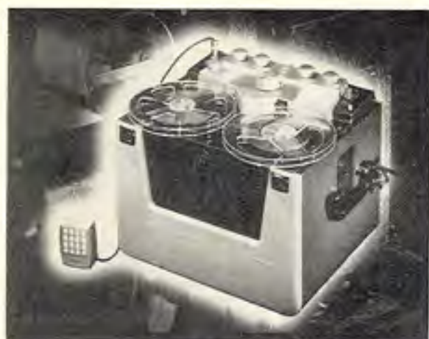
Left: the Revere Camera Company of Chicago developed its Synchrotape to permit more accurate synchronization of sound from tape with home movies. The tape was striped and the flicker of the projector shutter provided a stroboscopic light effect to time the recorder and projector. Adjustments in speed were made manually. Right: automatic control of slides for home and business was provided by this Model 207 Ekotape. The top track of the tape was used for voice or music and the lower track for signals which, through a relay, operated a slide projector and changed pictures without an operator touching the controls. Earlier devices included a photo cell mounted on a recorder which picked up the light reflected from white tabs attached to the back of the tape.
