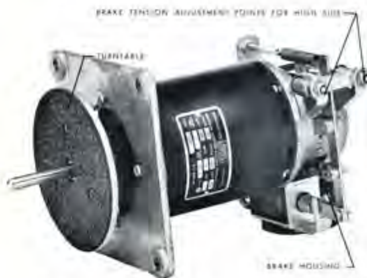
BRAKE ADJUSTMENT, HIGH SIDE
