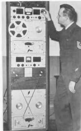
Recorder setup for the time-delay loop showing the two Magneorders, special panel with unison roller and amplifier which form the basis of method described by Lt. Jesse C. Durham, USNR, for AFRS "Editing without Cutting Tape."
