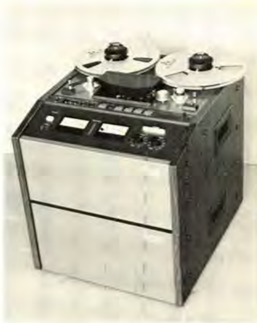
Figure 7. Two channel fixed-head PCM recording deck.
