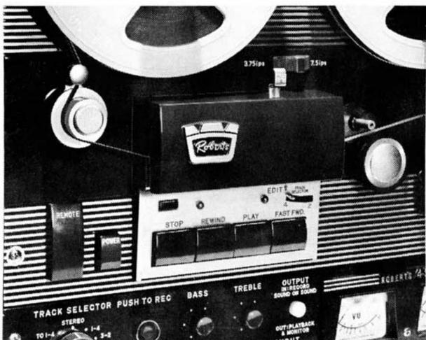
**MUTE CONTROL** — is used to push the tape from the erase, record and play heads during fast forward or rewind. This eliminates wear which could result from super fast motion of the tape across the heads.
