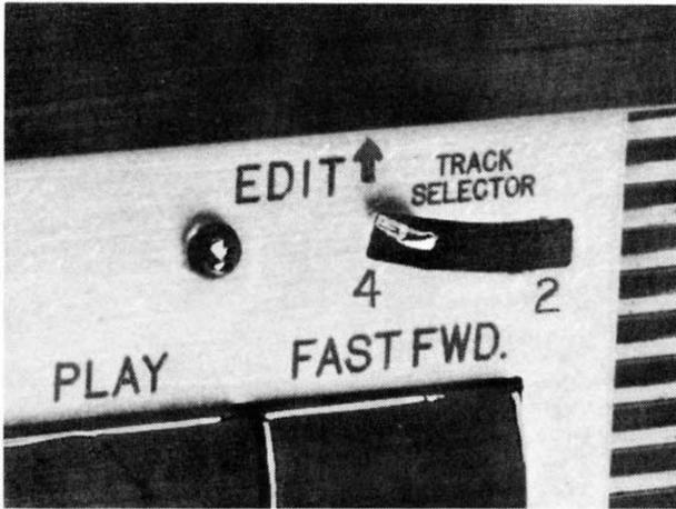
**TWO-FOUR TRACK SELECTOR** — The track selector switch is used to adjust and realign your playback heads to accommodate either ¼ track stereophonic or monaural pre-recorded tapes, (4 position) or 2 track (½ track) stereophonic or monaural pre-recorded tapes, (2 position).
