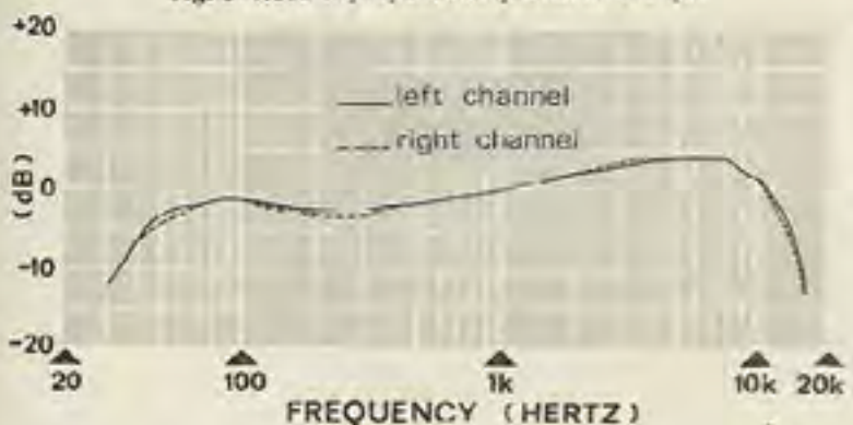
Fig. 8—Record/playback response at 3 3/4 ips.
