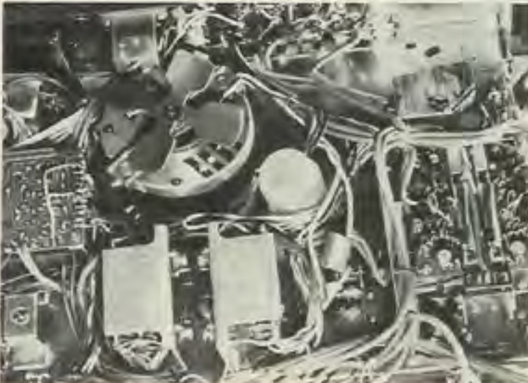
Fig. 5—The Sony 230's underside shows its electronics and motor. You can see the output transistors that are mounted in heat sinks in the bottom part of the photo, as well as a printed-circuit board at left.
