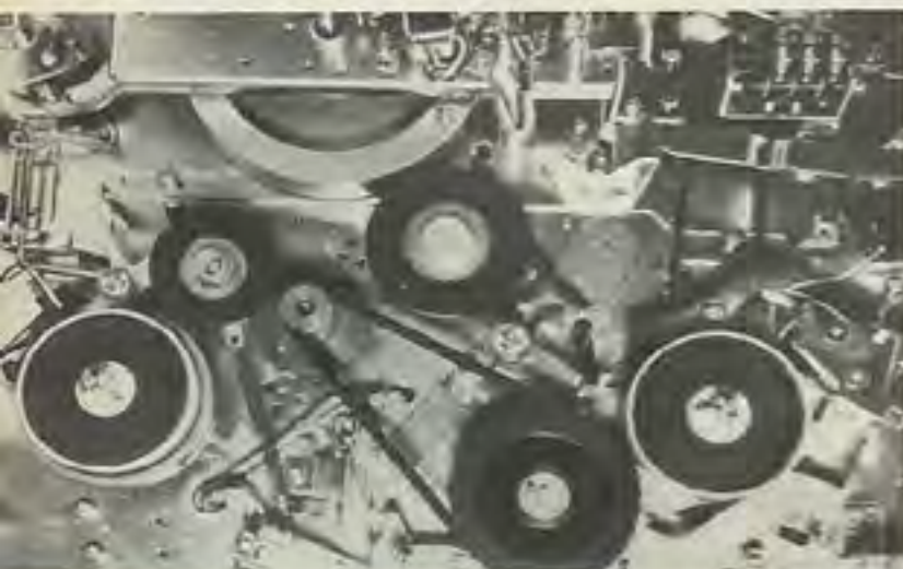
Fig. 2—The 230's drive mechanism is pictured here. In rewind position, the outside of a band of rubber around the idler drives a clutched supply turntable. For fast-forward drive, the small rubber idler is driven by the outside band of rubber around the motor pulley.
