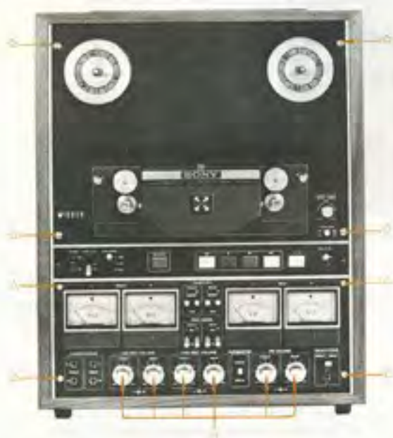
Fig. 2-1. Reel panel and amp panel removal
